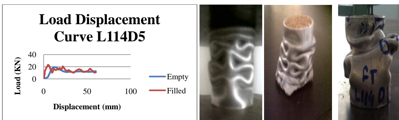
Load Displacement Curve for L/D=3 at 5°
